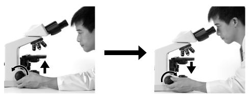
Raise the stage until this distance is slightly smaller than the working distance.
