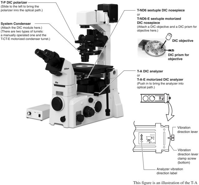
This figure is an illustration of the T-A DIC analyzer. For an illustration of the T-A-E motorized DIC analyzer, please refer to the instruction manual supplied with the T-HUBC HUB controller.
