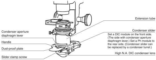
Loosen to move the slider back and forth.
