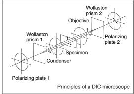
After the two rays pass through the specimen, they are collected by the objective onto the back focal plane of the objective. Wollaston prism 2 is placed here to recombine the two rays back into one. However, the rays do not interfere with each other since they have perpendicular planes of polarization.
