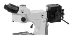
Mercury lamp house fitted in place
