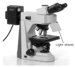
Light shield fitted in place
