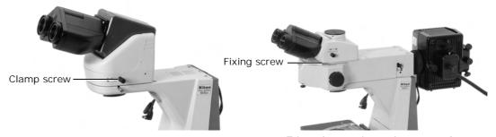
Trinocular eyepiece tube mounted on the fluorescent unit
