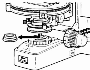
The analyzer can be rotated by first loosening the analyzer clamp screw **1** and then turning the rotation dial **2**. The angle of rotation can be read to 0.1 degrees over a range of 0-360 degrees with the vernier.
