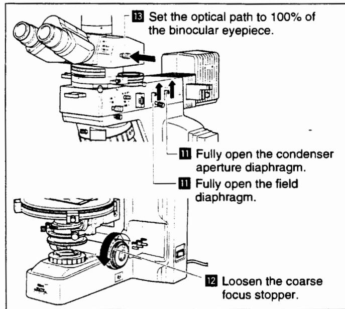
**14** Turn the diopter adjustment ring of the right eyepiece (containing the crosshairs) and focus on the crosshairs.
