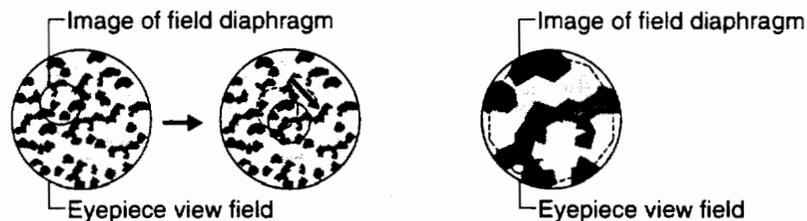
Focus and center the condenser so that the light passing through the condenser forms the image at the correct position on the specimen (i.e., at the center of the optical path).
