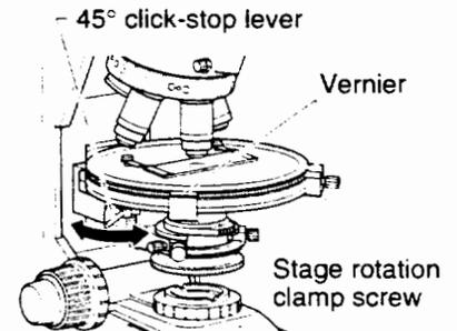
Release the click-stop device where the stage has dropped into a click position. If the click-stop device is released where the stage is not at this position, the first 45° increment will not be accurate the next time the click-stop device is operated.
