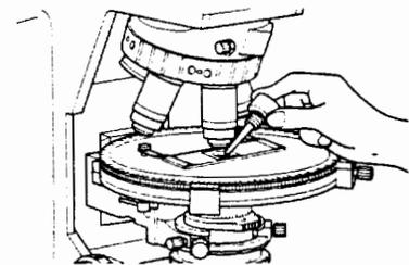
Any oil remaining on an oil-immersion type of objective or staining on the tip of a dry type of objective has a negative effect on viewing. After using oil, wipe all of it away and make sure that there is no oil on the tips of the other objectives.
