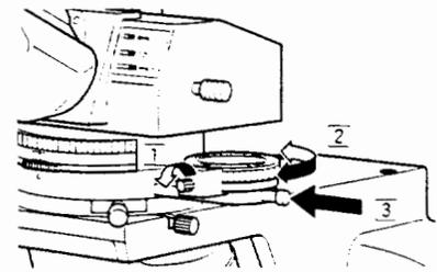
Since the intermediate tube contains a built-in depolarizer, it is not necessary to be concerned about the relationship between the orientation of the polarizing plate and photomicrographic devices.
