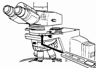
It is normal to bring the top lens of the condenser into the optical path when observing at a magnification of 10× or greater. Measuring the retardation or evaluating by interference color, however, stop down the condenser aperture diaphragm or swing out the top lens even for a magnification of 10× or higher (with the aperture diaphragm fully opened), and illuminate with light that is as parallel to the optical axis as possible.
