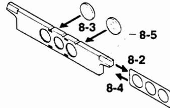
The eyepiece tube, intermediate tube and epi-illuminator are provided with positioning pins, while the intermediate tube, epi-illuminator and microscope arm are provided with grooves for engaging with those pins. Remove any looseness between the pins and grooves that occurs during assembly by pushing in on the component provided with the pin while turning in the clockwise direction.
