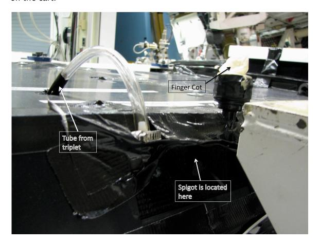
View you see when the spectrograph is mounted on the telescope. Spigot is located above the "OPEN CLOSED" label.
