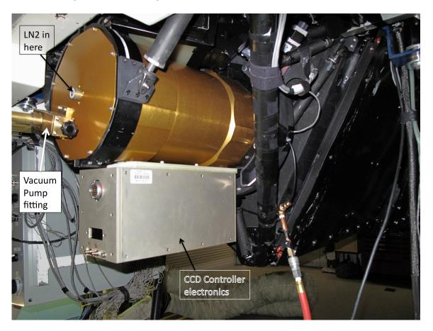
The dewar being filled. MAESTRO is on the cart. A piece of aluminum has been placed on top of the "MAESTRO CCD Fill" PVC to further protect the vacuum fitting.
