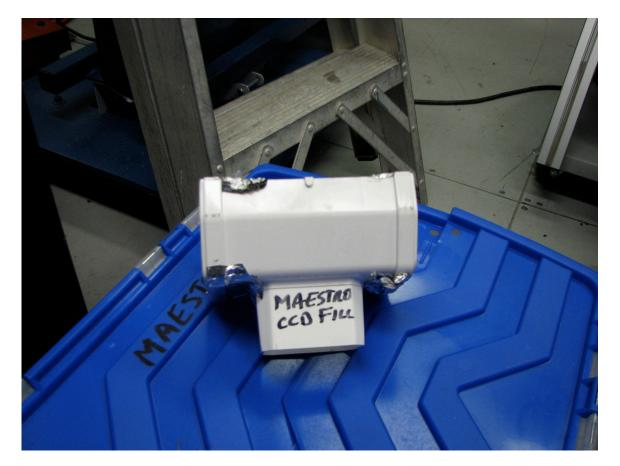
The anatomy of the dewar, showing the hole for LN2, and the vacuum pump fitting. The spectrograph cover has been removed in this picture.
