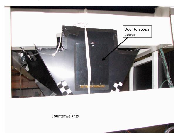
The PVC fixture used to protect the vacuum fitting from damage while filling the dewar:
