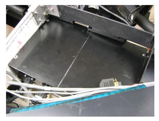
The comparison box cover has been removed showing the inside of the box. This is an old picture, taken during construction, and the filters have not yet been mounted. The picture was taken from the grating side of the spectrograph, so the box appears upside down compared to the pictures above.
