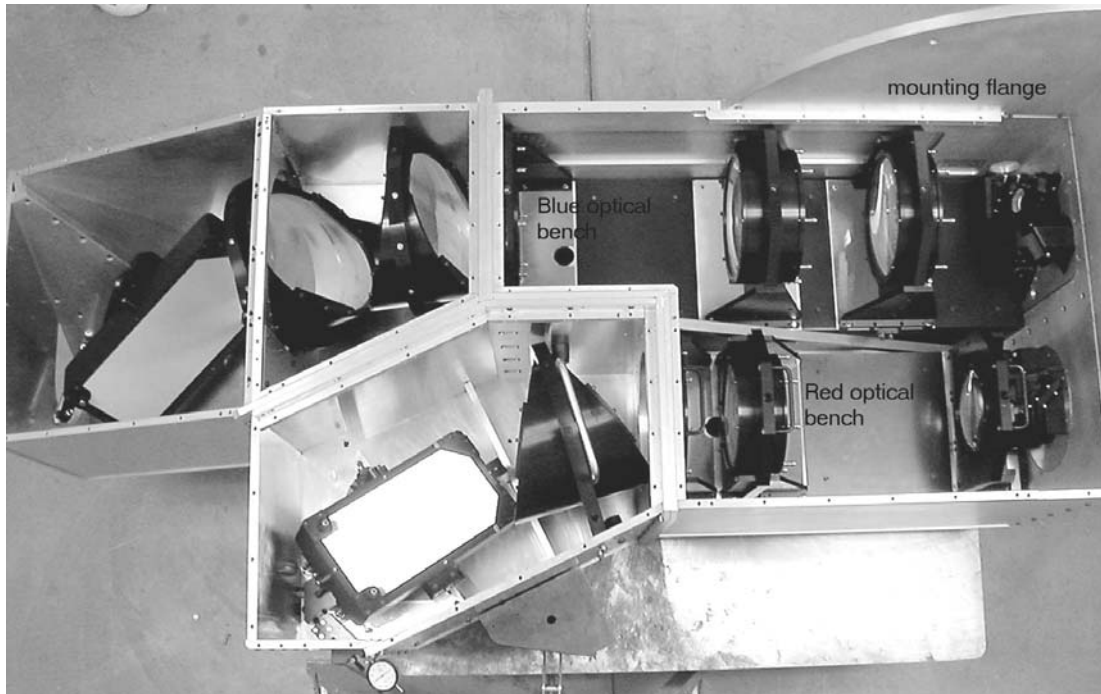
Figure 2: Top view of MIKE with covers off. The main box contains the red and blue optical benches (labeled). The blue box contains the 2 blue prisms and the R2.6 grating (towards top left corner). The red box contains the red prism and R2 grating (lower left). Light comes from the telescope through the mounting flange at the top right of the photo.
