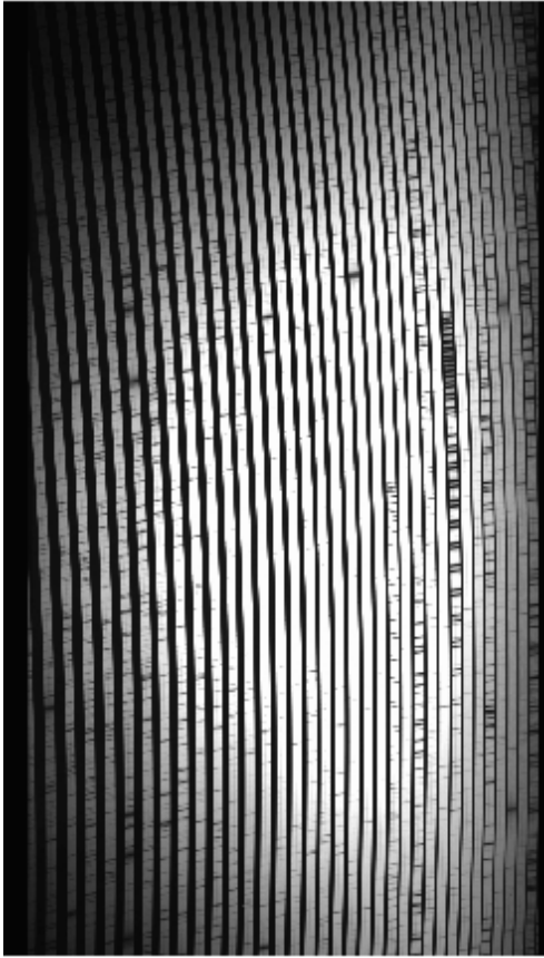
Figure 15: A solar spectrum taken with the red side through the 0.5 x 5 arcsec slit.
