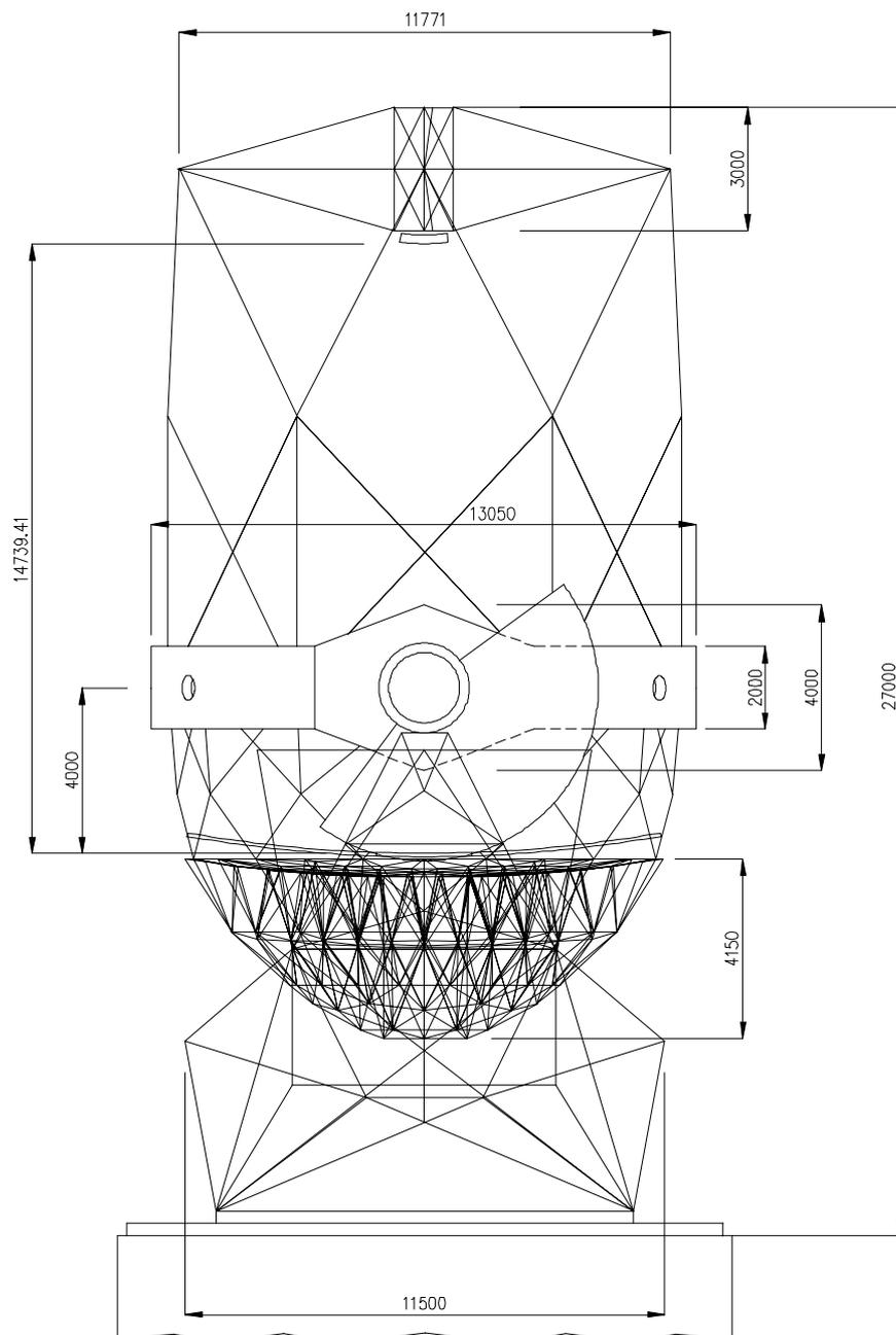
Figure 5.3: Lateral (y-z) view of telescope structure (dimensions are in mm).
