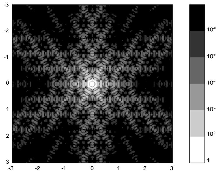
Figure 4.8: Diffraction image of a mirror with hexagonal segmentation of 36 segments. The intensities are normalized with respect to the maximum intensity. The scale is in units of  $\lambda/a$ ,  $a$  being the side of one of the hexagons. The diffraction limit of the mirror is approximately  $\lambda/6^a$ .
