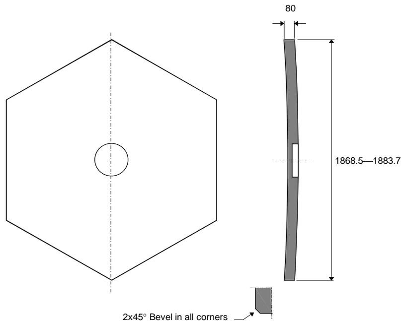
Figure 4.9: Primary-mirror segment blank (dimensions are in mm).
