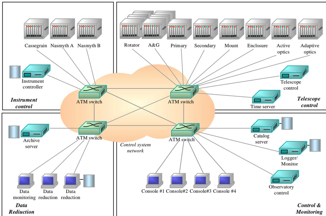
Figure 8.8: Hardware architecture.
