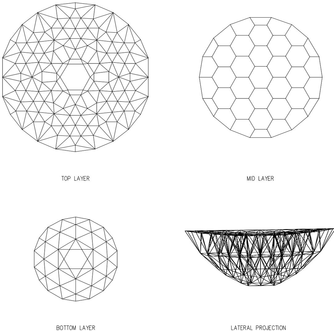
*Figure 5.5: Primary-mirror cell structure.*
