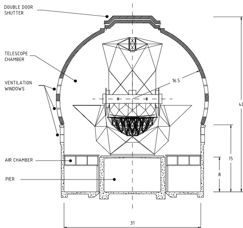
Figure 6.3: Selected dome type (dimensions are in m).
