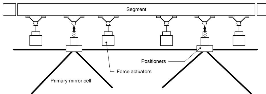
Figure 4.11: Axial support using active generation of support forces.
