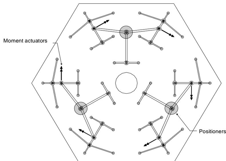
Figure 4.10: Axial-support whiffletrees (arrows show the axes of the moment actuators).
