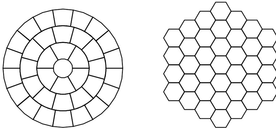
Figure 4.7: Plan view of circular and hexagonal segmentation.
