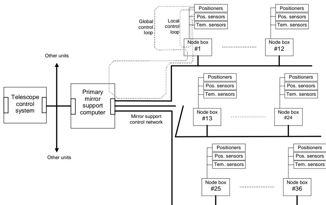
Figure 4.13: Control-system network showing the route of the global and local control loops.
