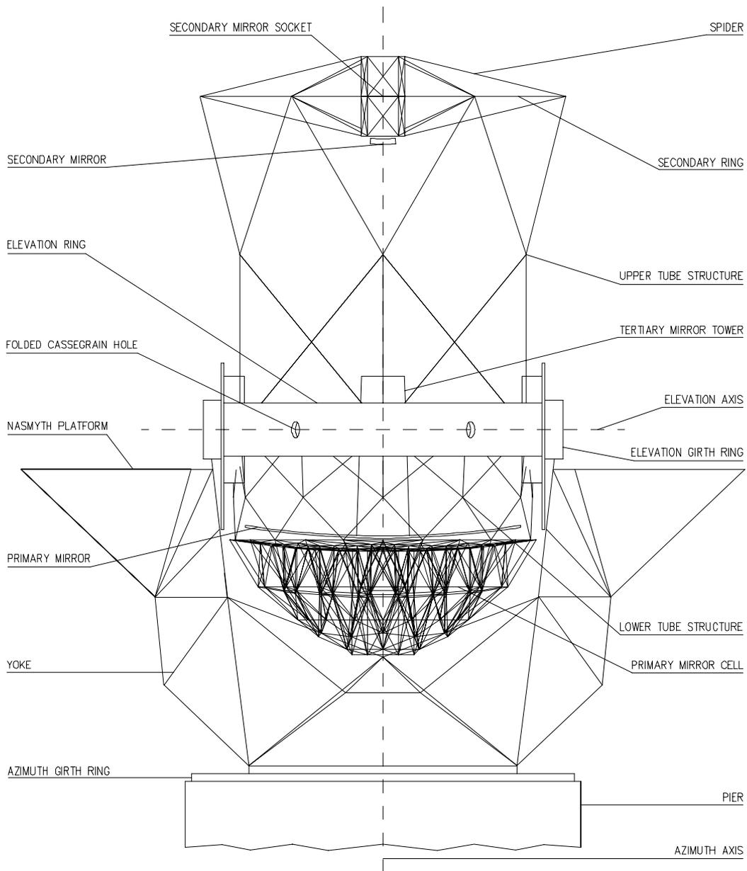
Figure 5.4: Subsystems of the telescope.
