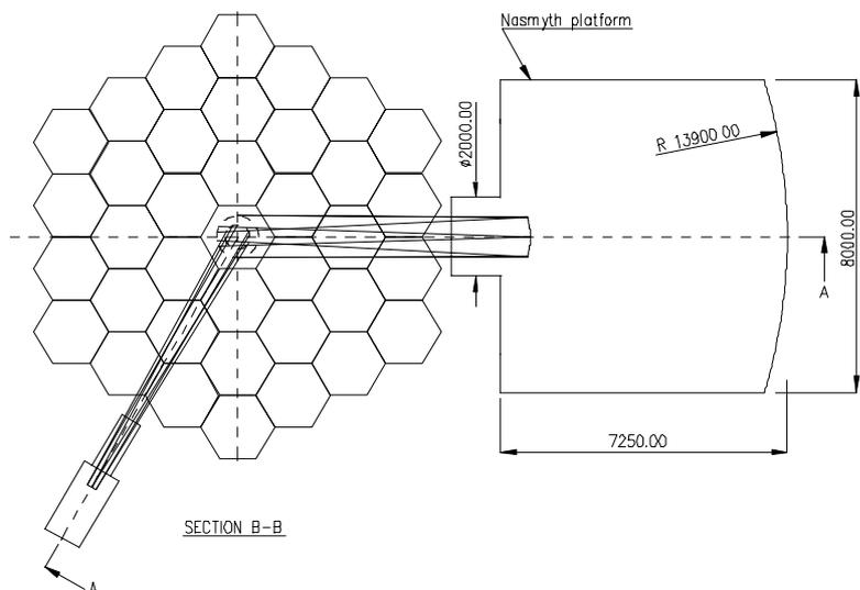
Figure 5.1: Layout of GTC ray path and foci (dimensions are in mm).
