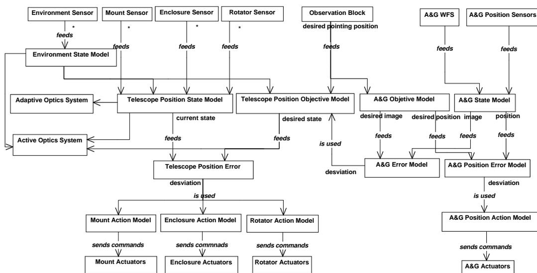
Figure 8.3: Telescope position control class diagram. An explanation of the different models used to represent the domain of the problem can be found in Section 8.5.2.2.
