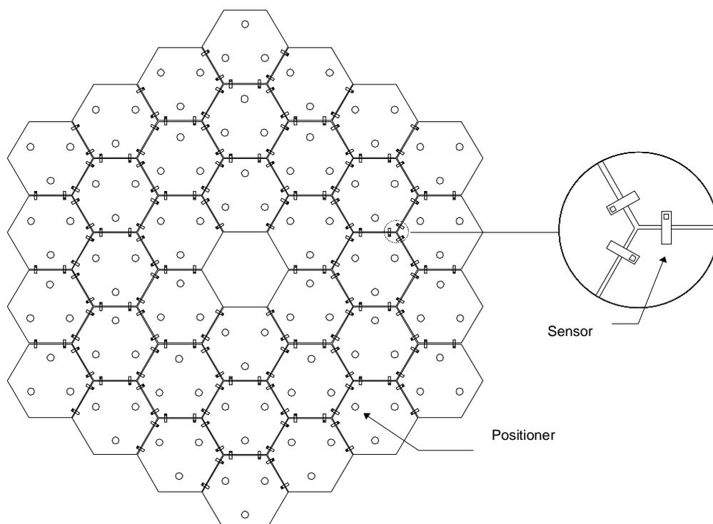
*Figure 4.12: Plan view of the distribution of the segmented primary mirror showing the positions of sensors and actuators.*
