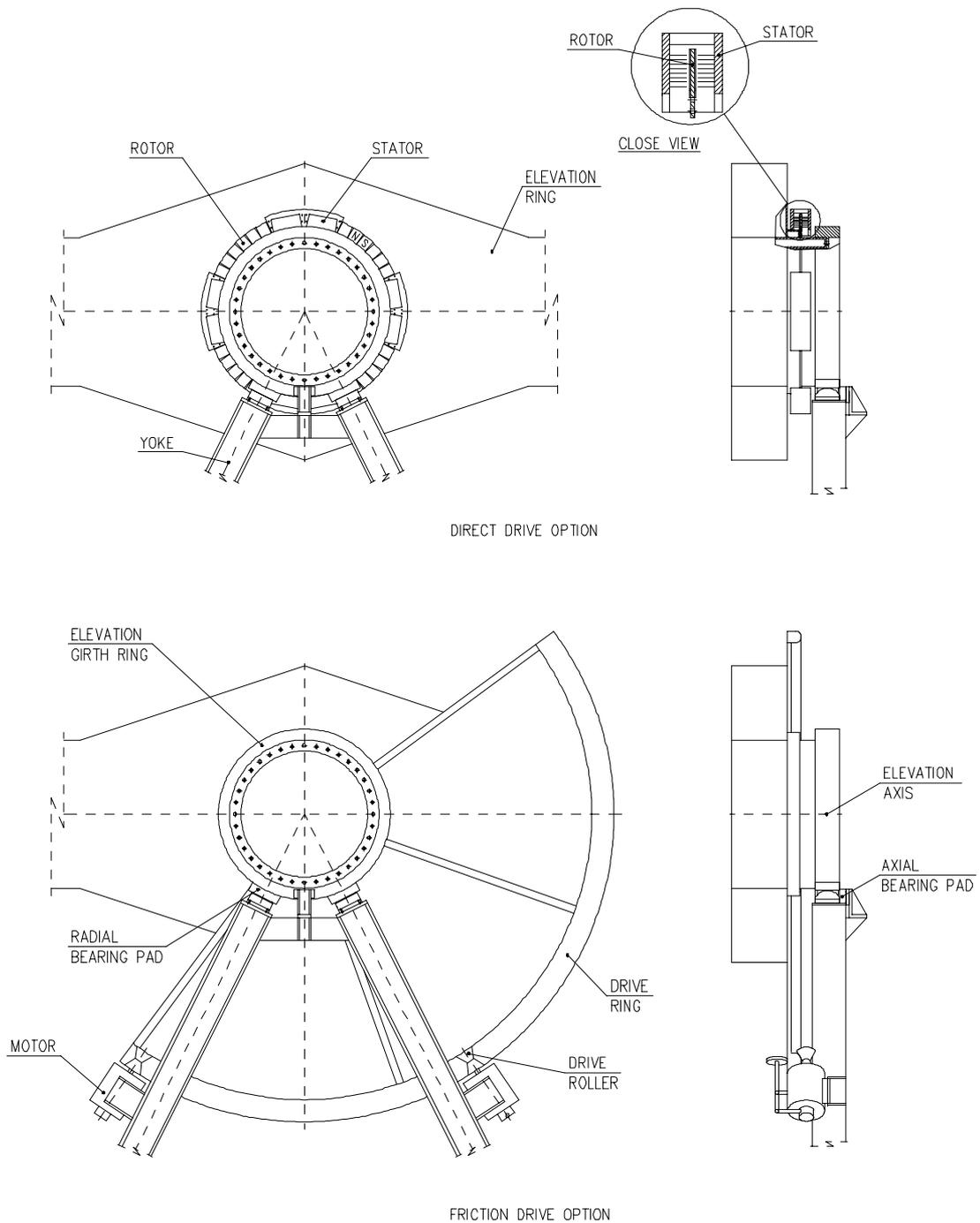
Figure 5.7: Hydrostatic bearing arrangement and drive options for the elevation axis.
