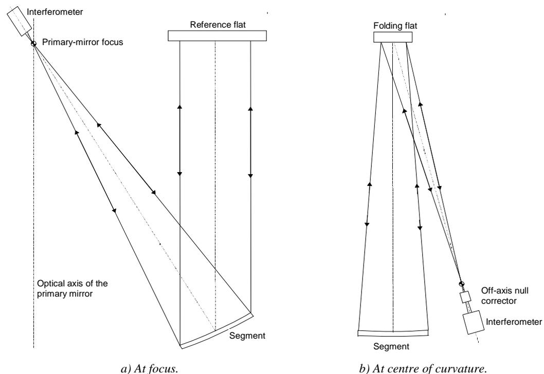
Figure 4.14: Interferometric test of the segments.
