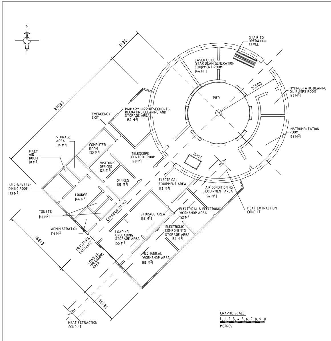
Figure 6.5: Plan view of the installation, showing a tentative distribution of the support areas.
