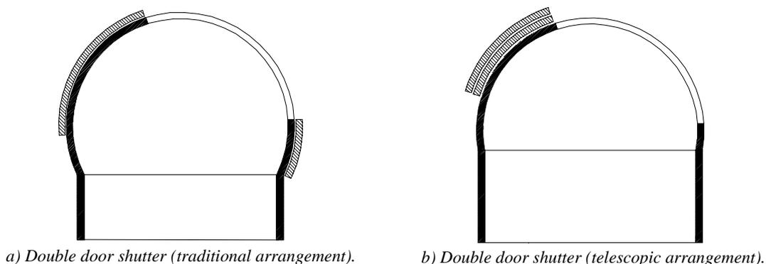
Figure 6.4: Alternatives for the dome shutter.
