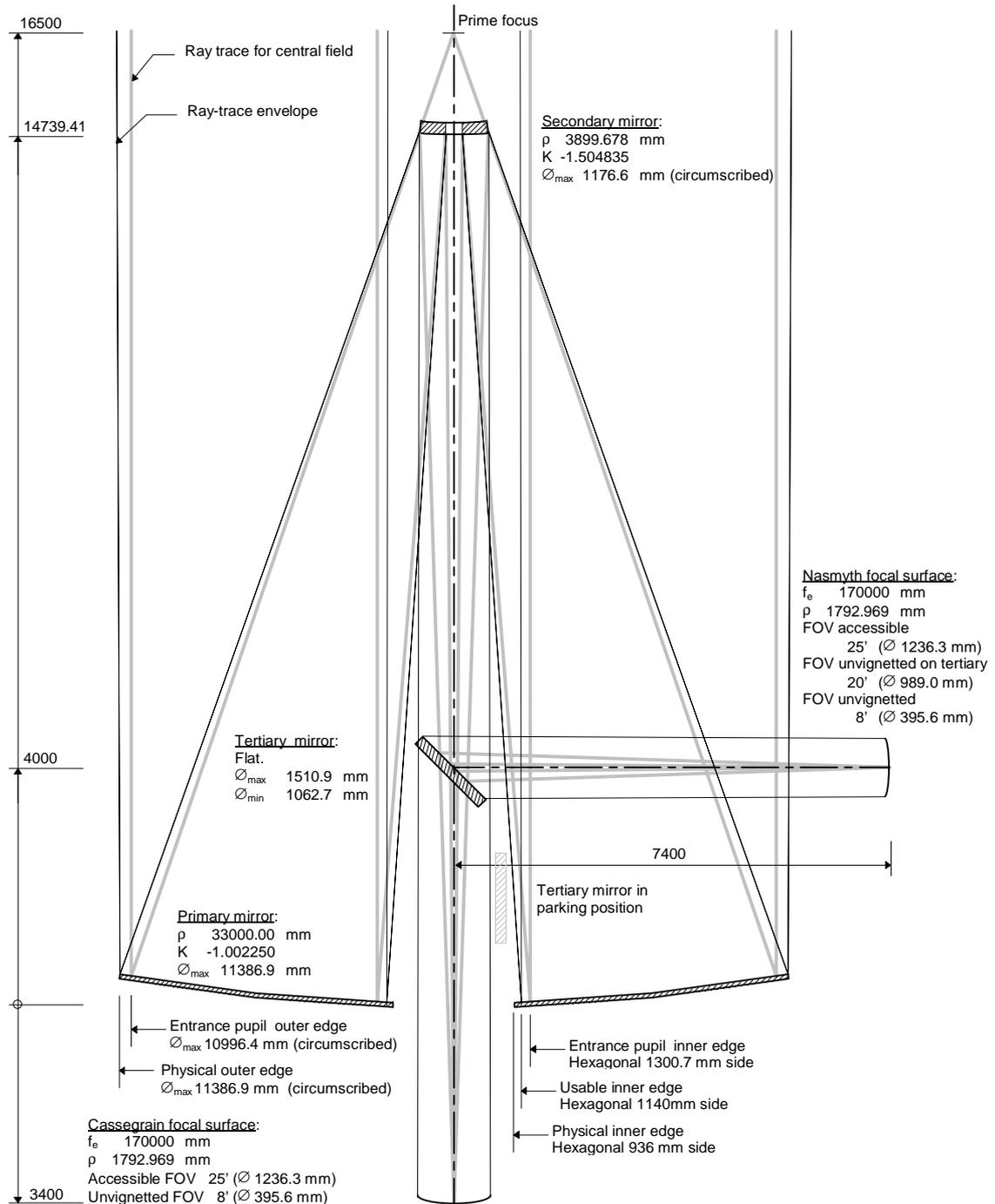
Figure 4.2: Optical configuration of the GTC (dimensions are in mm).
