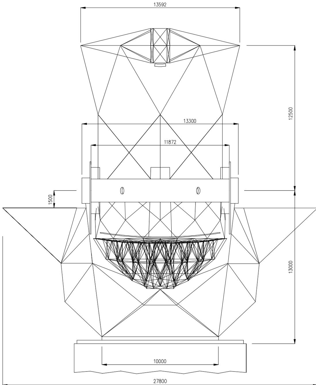
Figure 5.2: Frontal (x-z) view of telescope structure (dimensions are in mm).
