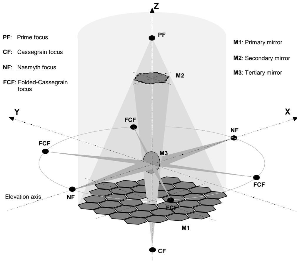
Figure 4.1: Optical system and foci.
