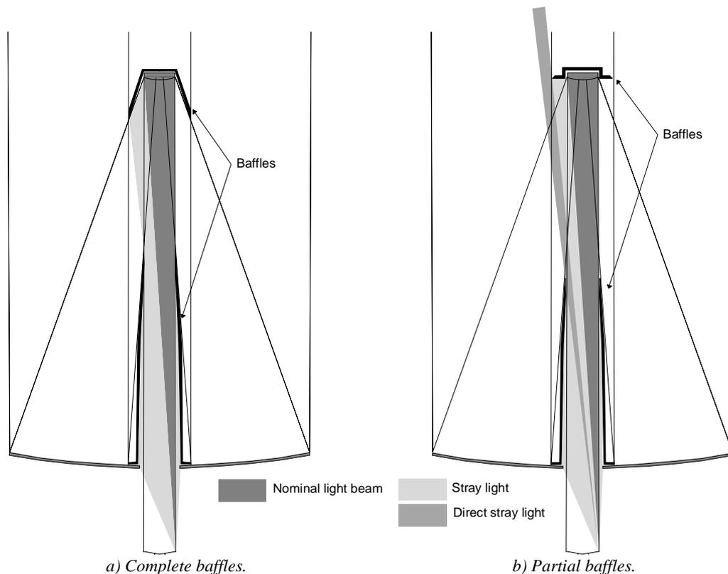
Figure 4.5: Telescope baffle system.
