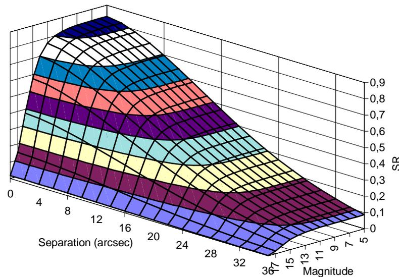
Figure 4.6: Strehl ratio at  $2.2 \mu\text{m}$  as a function of magnitude and separation of natural guide star for a system with 250 actuators/subapertures.
