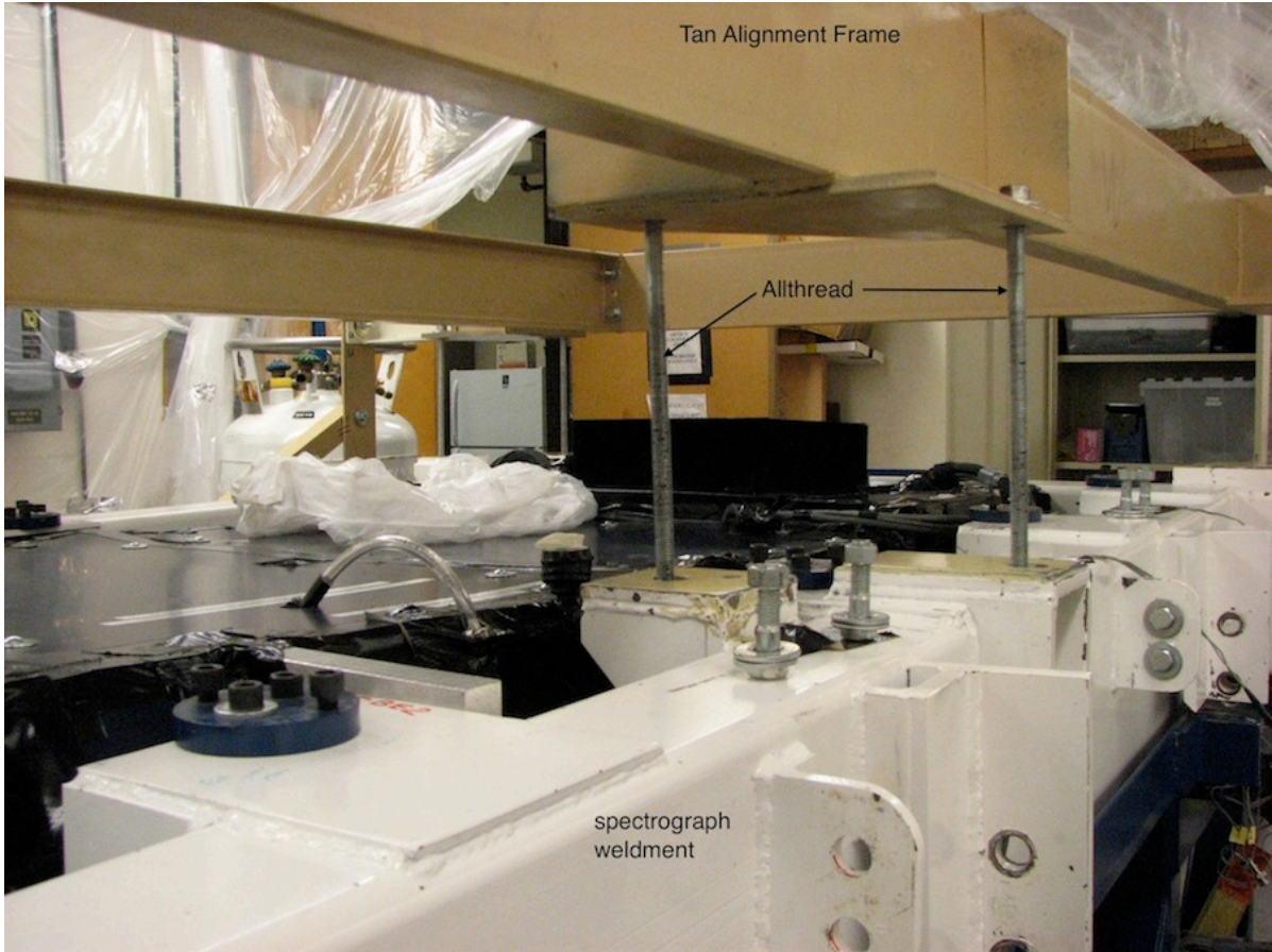
White spectrograph weldment is hanging from the tan alignment frame by allthreads during raising/lowering of spectrograph from the cart. Two of 6 total allthreads are labeled.
