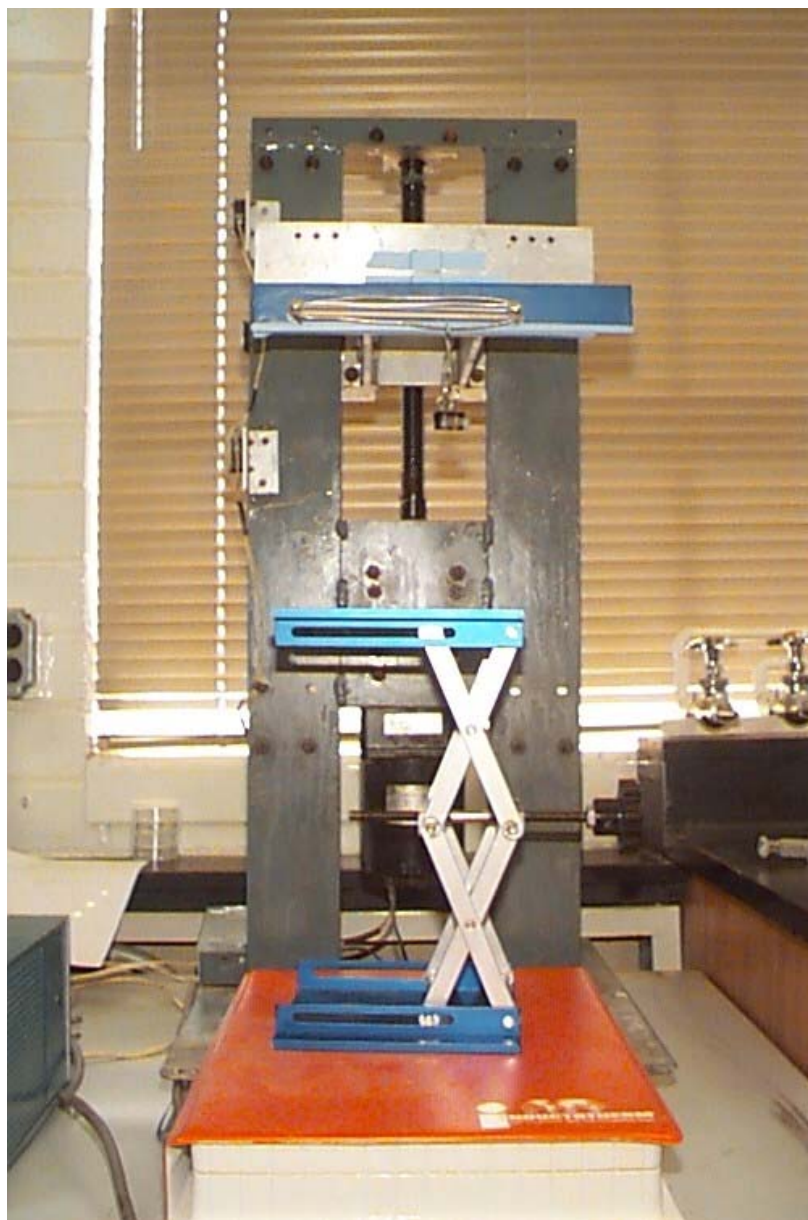
FIGURE 5.5. Closer look at dipping apparatus. Paperclip is sample holder.
