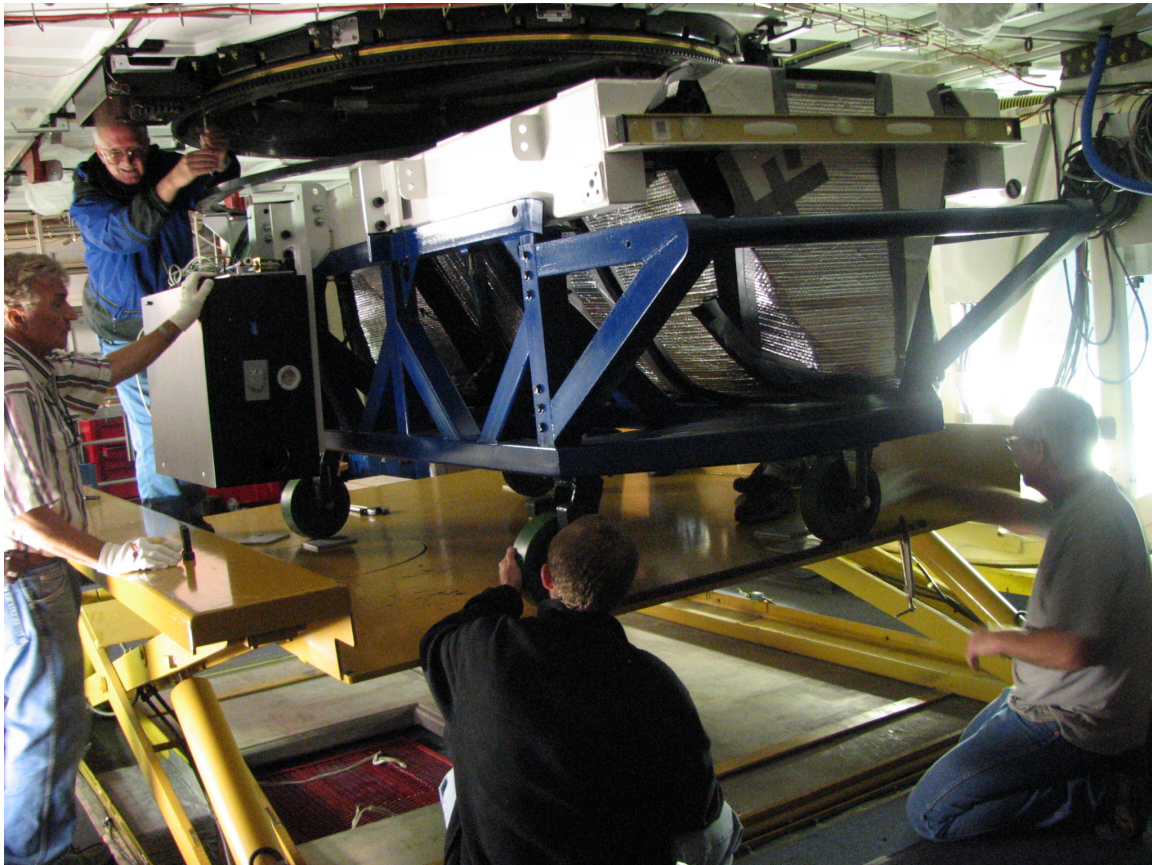
MAESTRO on the instrument lift. The stop bar, in the foreground, is attached to the lift with a c-clamp.
